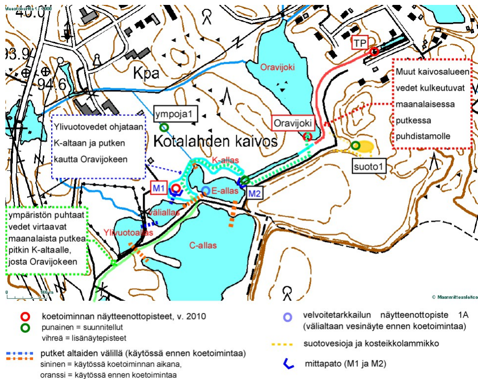
Figure 18: Water arrangement and measurement pond locations in the 2010 trial (photo, Groundia Oy 2010 trial plan.)
